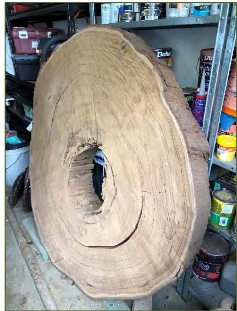
Figure 46 The unprocessed and remaining portion of the trunk sample after the removal of the section for ring analysis.
