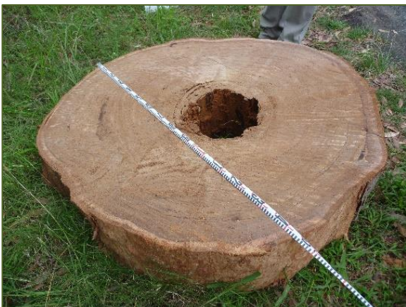
Figure 26 The salvaged disk was 230 mm thick...
