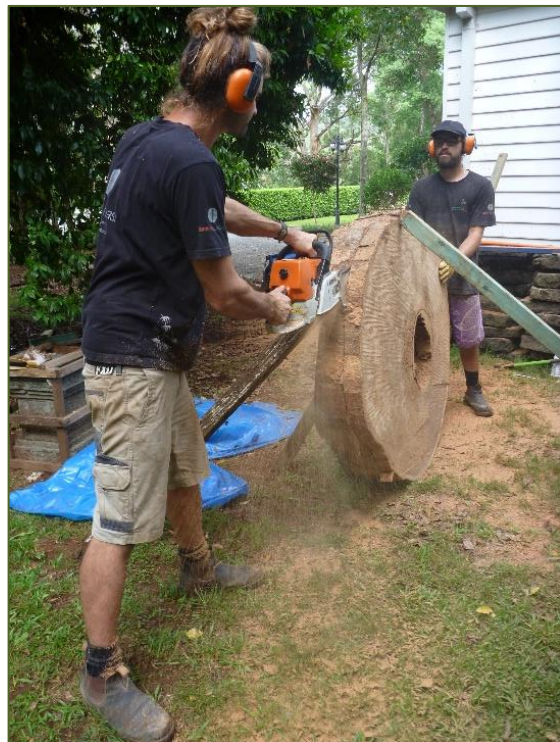
Figure 24 Cutting a 50 mm slice from the sample for tree-ring analysis (Clint Bramston left, and Jo Winkler right)
