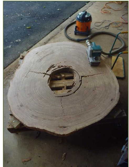
Figure 11 The sample after completion of the 80 grit sanding. Note the belt sander and use of a vacuum to capture the dust.
