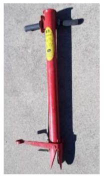
The Pottiputki can reduce bending when planting by sliding tubestock down the barrel of the device. Photo Ruth Aveyard
