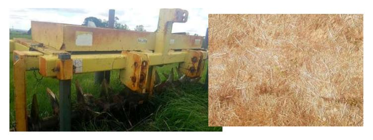
The aerator implement and the deep impressions created when used with the correct amount of soil moisture. Photo: Ruth Aveyard
