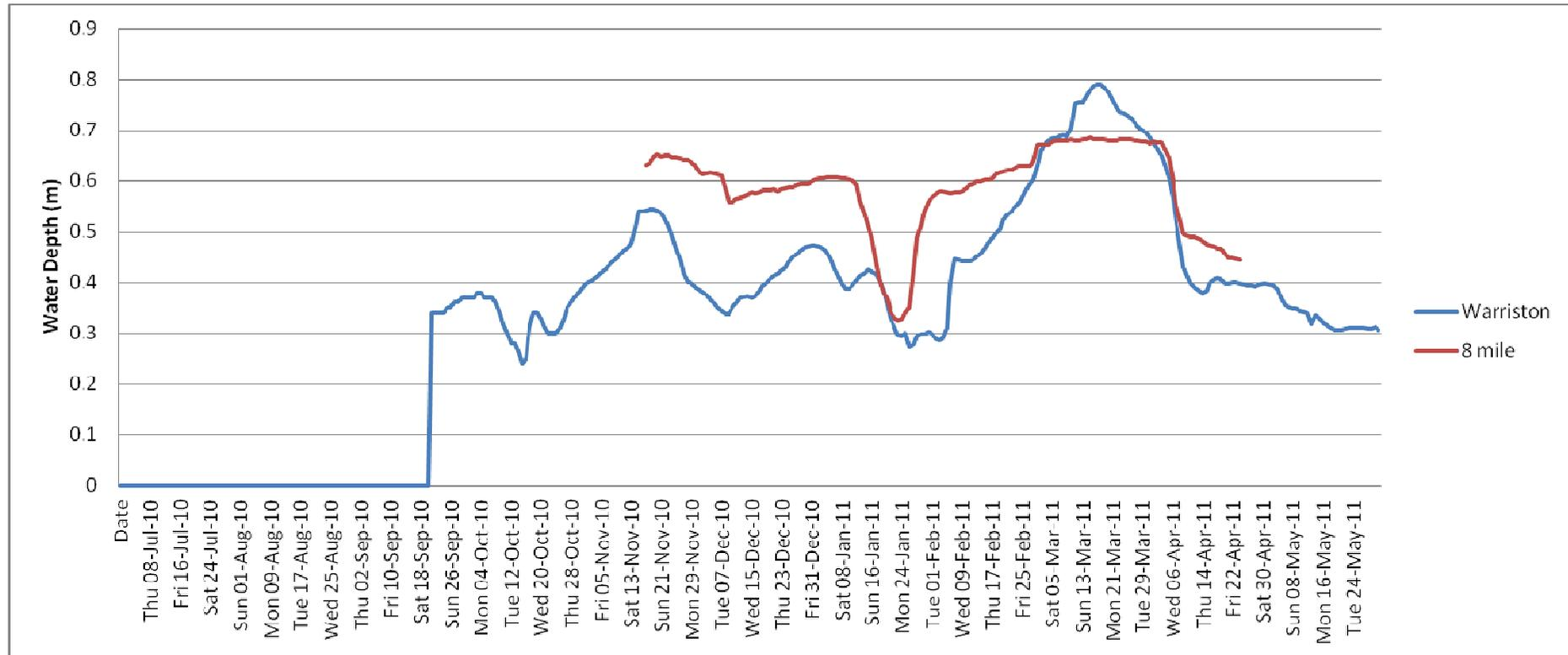
Figure 7: 2010/11 flood event showing the relationship between flows over Warriston Weir and water depths on the Eight Mile Creek road bridge (Cobb Highway) with a 20 day lag
