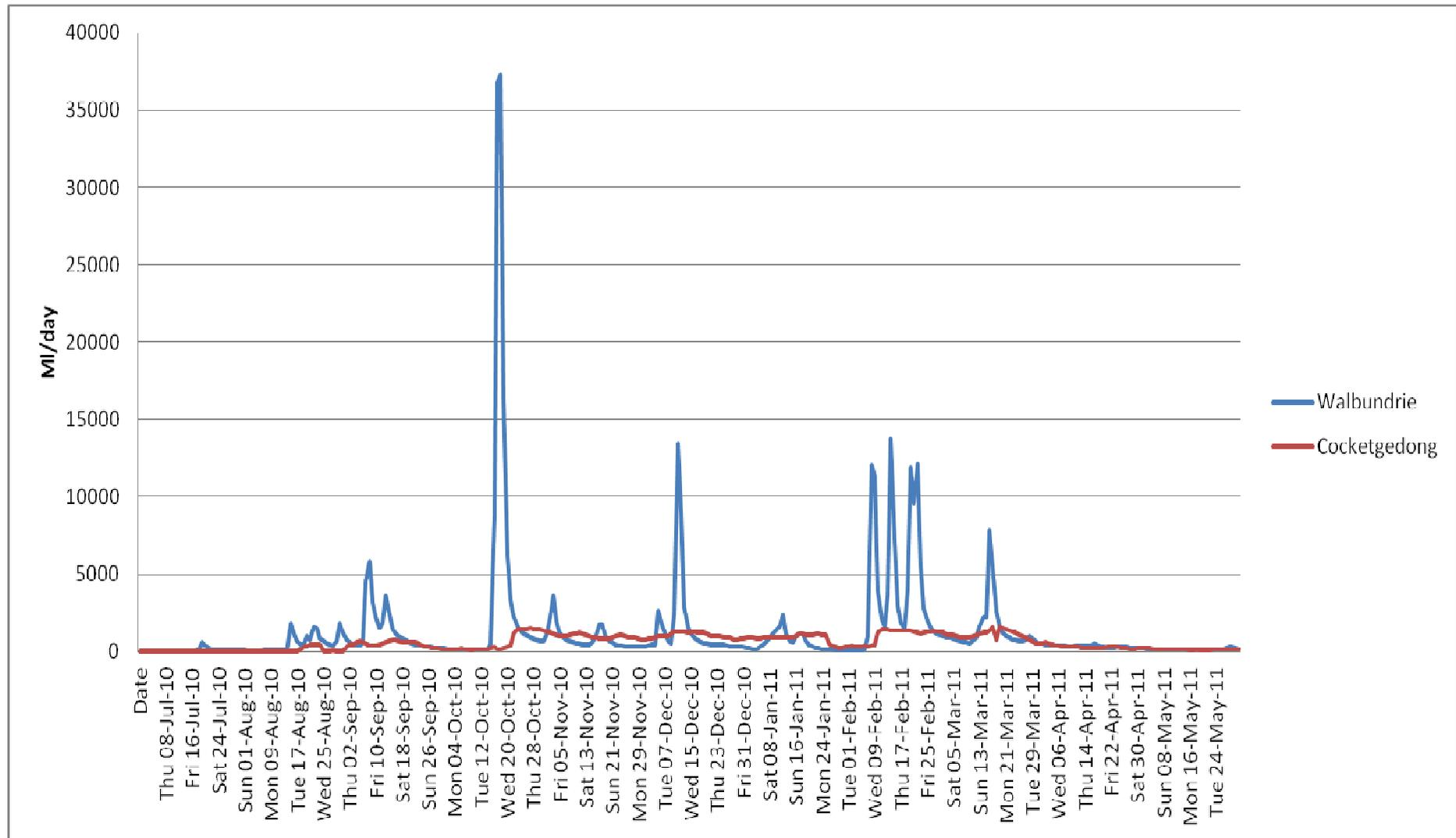
Figure 4: 2010/11 flood event - Walbundrie flow gauge compared to Cocketgedong flow gauge
