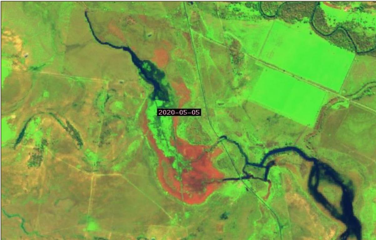
Figure 4: Sentinel 2 satellite image 5/05/2020 showing the site at maximum inundation extent and vegetation response to rain fall events in April and May (Sentinel Hub)
