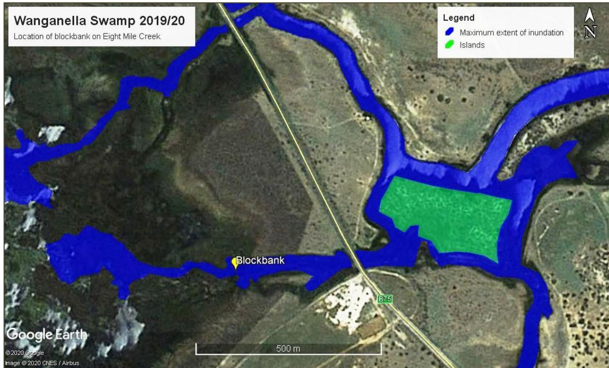
Figure 16: Location of the old block bank impeding flow via the southern Eight Mile Creek channel (Google Earth).
