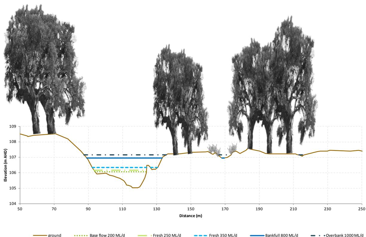
**Figure 26.** Cross section of the Middle Yanco Creek hydraulic model (XS 545) showing the environmental flow recommendations and habitat inundation
