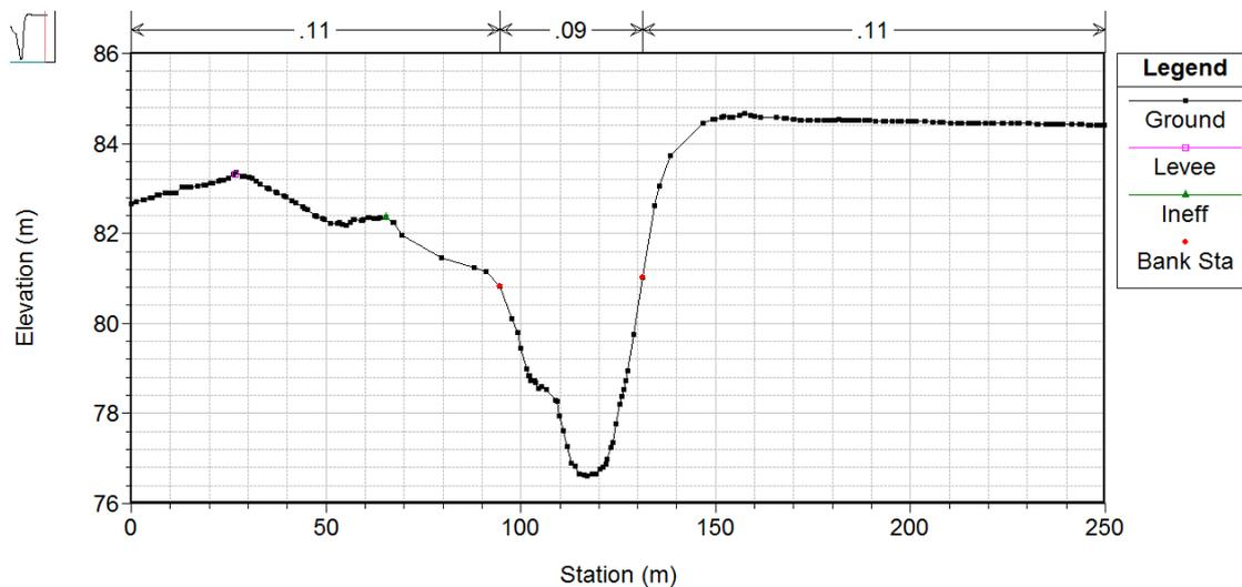
**Figure 16.** Survey cross section (lower Billabong Creek, chainage 623) showing feature survey to top of bank (note concentration of points in low flow channel and benches as compared to channel banks) and supplementary LiDAR survey into the floodplain.
