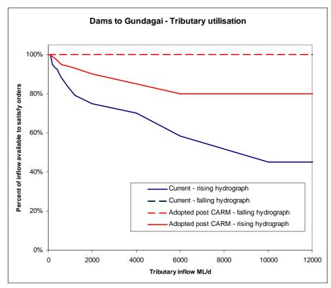
Tributary catchment rainfall runoff models will allow CARM to increase the amount of tributary flow used to fill downstream orders, particularly on the rising limb of hydrographs. In both cases IQQM assumes 100% utilisation on the falling limb. Depending on the calibration accuracy of the rainfall runoff forecast models, CARM IQQM predicts and utilises up to 80% of rising limb flows to allow for a more realistic forecasting improvement.
