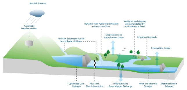
CARM is making control of water flows and dam releases more precise and efficient through linking the physical upgrades to river infrastructure and accurate measurement/metering with hydrodynamic operational modelling and flow information systems.
