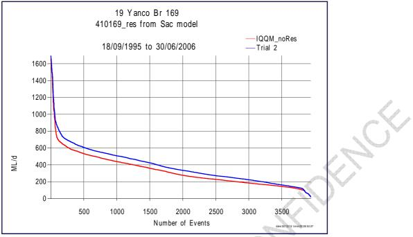
Figure 4 410169 – Flow duration curve, Observed data, Simulated without residual flow and simulated with residual from Sacramento model Trial 2
