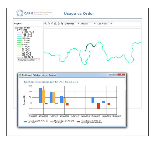
This dashboard plot indicates the orders and usage difference (negative) in the section Murrumbidgee Ch 713 to Ch 761, ie. more water has been pre-ordered than extracted. This could be due to a rainfall event, or a poor ordering regime in this section.
