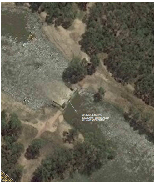
Figure 29. Proposed upgrade to arrangement at Yanco Regulator
