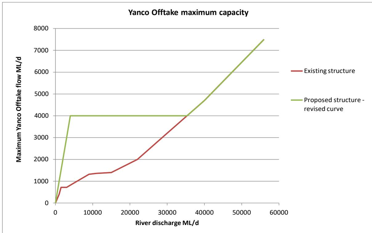
Figure 1 Yanco Offtake existing and post-project maximum capacity rating
