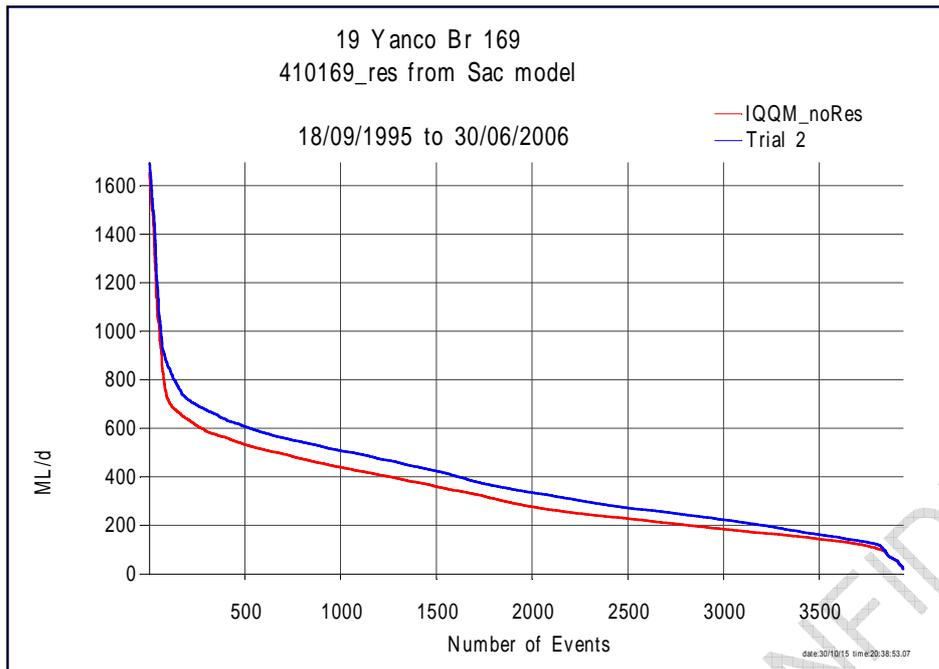
**Figure 4 410169 – Flow duration curve, Observed data, Simulated without residual flow and simulated with residual from Sacramento model Trial 2**
