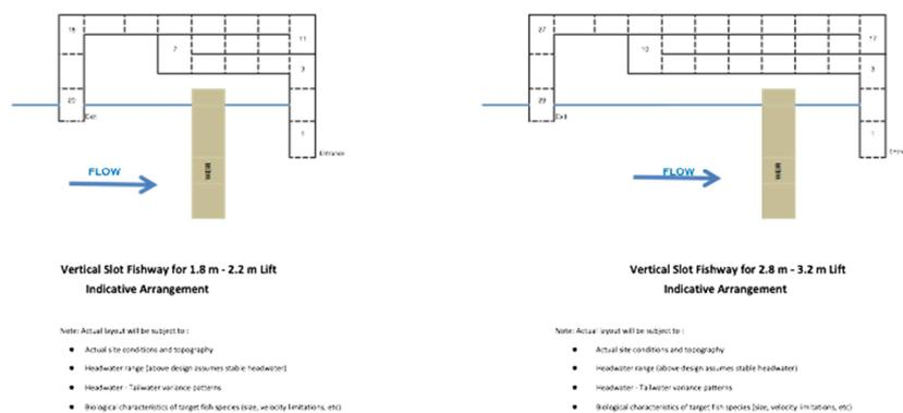
**Figure 3-5: Standard vertical slot fishway**
