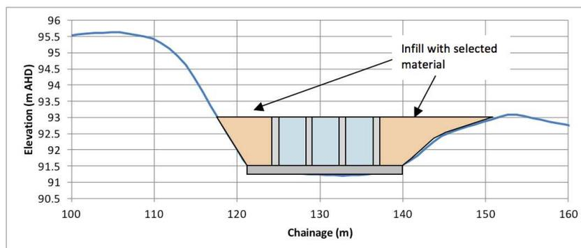
**Figure 3-2: Configuration of gates overlaid on cross-section at nominated site.**
