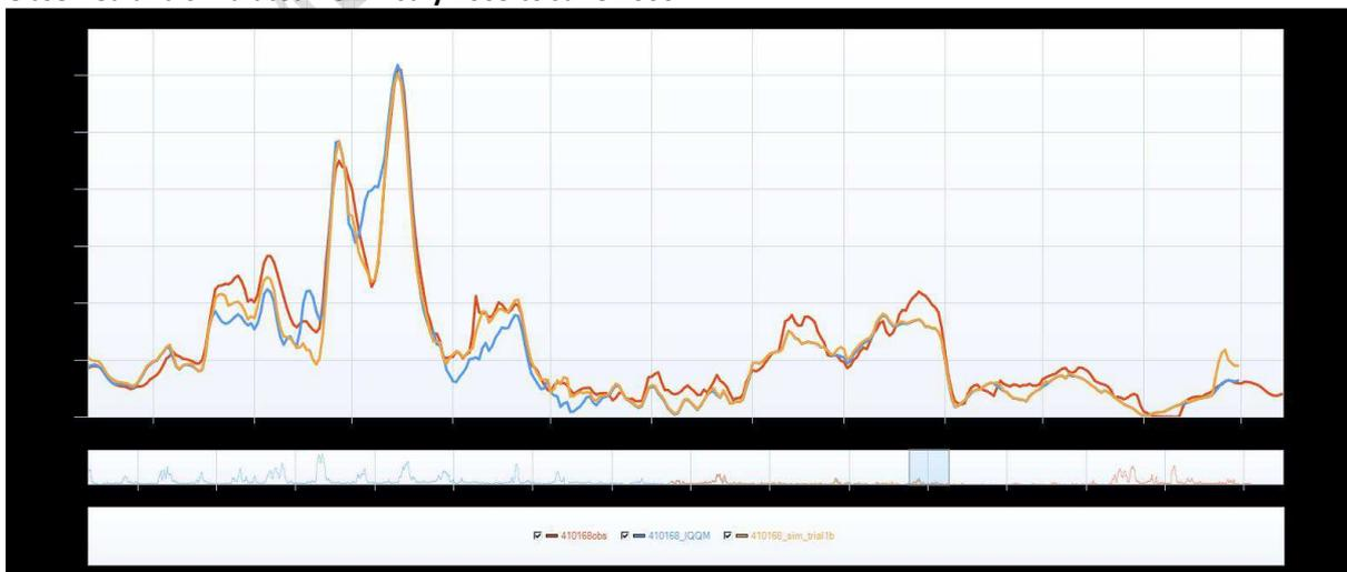
Reach 7 Time series plots of observed flows at 410134 (red line), 410134\_R3\_7 (blue line, simulated flows from IQQM reach model) and Trial 2 (orange line)
