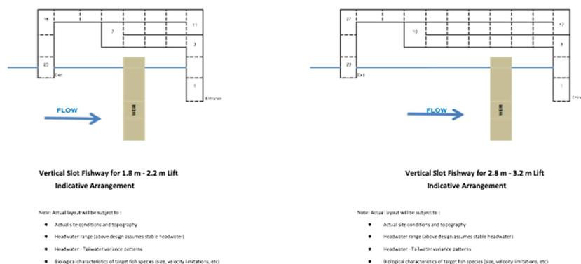
**Figure 3-5: Standard vertical slot fishway**
