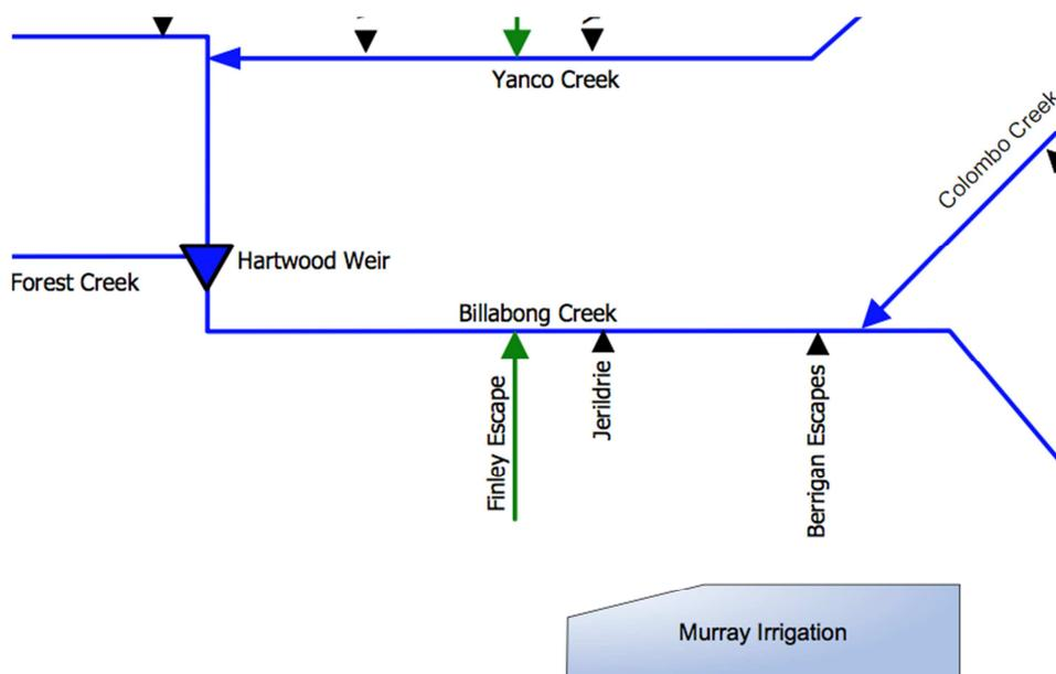
The existing agreement gives WaterNSW access to 250ML/day as a second priority supply. The proposal is to upgrade this agreement to deliver up to 300ML/day into the Billabong Creek, with the same rights as a standard customer. This would provide the major source of supply for diverters in the lower half of the system on the mid Billabong Creek, Forest Creek and lower Billabong Creek, past the junction with Yanco Creek.
