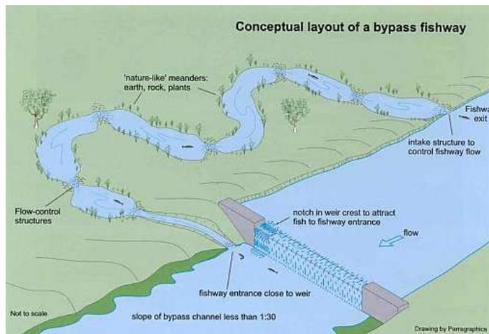
**Figure 3-4: Conceptual layout of a bypass fishway**
